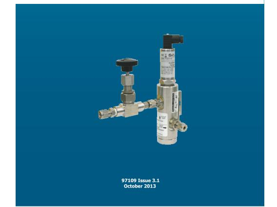
The Easidew Sampler is a modular low-cost, self-contained, filtration block and flow control arrangement which is suitable for any Michell impedance dew-point transmitter with 5/8" - 18 UNF process connection size, and is able to perform dew-point measurements at 200 barg (2900 psig).
